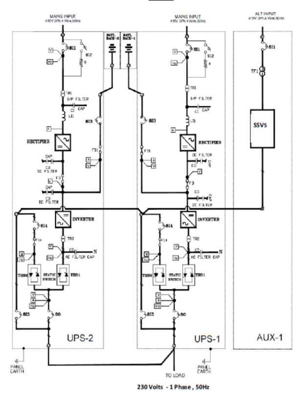
3 Phase input- Single Phase output, 60 KVA online UPS with inbuilt Isolation transformer including battery bank for minimum 30 minutes back up to be supplied strictly as per the above electrical diagram.
