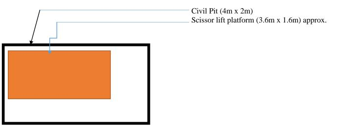
Note: 400 mm gap (two sides) in the pit left for maintenance purpose. After installation of scissorlift by the successful bidder, the remaining pit 400 mm on both sides will be covered with Chequered plate by BRBNMPL.
