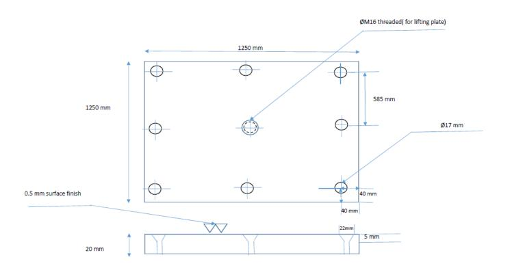
Note: The MS Plate should be milled on top surface with smooth surface finish and the flatness in the total machines area should be within 0.5mm
