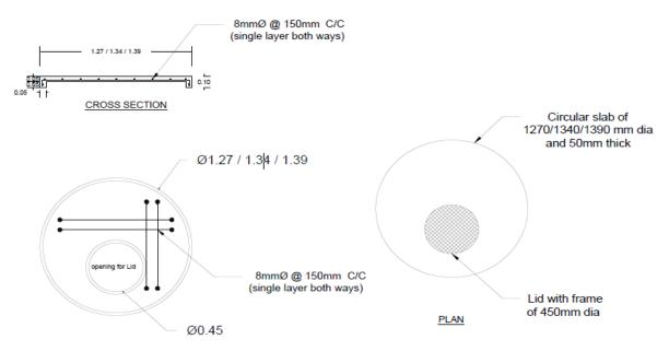
REINFORCEMENT DETAILS OF SLAB
